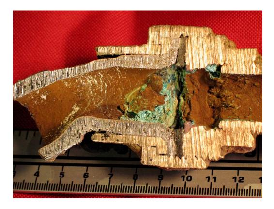
Build up of excess scale at the junction between Pb pipe and brass fitting. The brown scale to the left is dominantly  $PbO_2$  with some white Pb carbonate underneath, whereas the scale to the right, on the brass, is dominantly Mn oxide. At the junction, Cu sulfate dominates.
